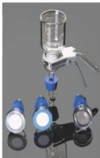
Filtration Glassware, Glass Filter Holder For 47 mm Disc Filters
